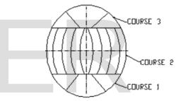
Fig. 5. 3-Course Version Spherical Vessel
